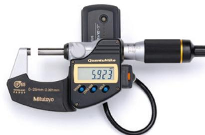
Electronic data collection allows the user of the gage to send the measurement displayed on the gage directly to a computer by simply pushing a data send button. An incredible variety of Data Management is available. From USB cables and multiplexer systems to wireless systems, MeasurLink® can support them all.
